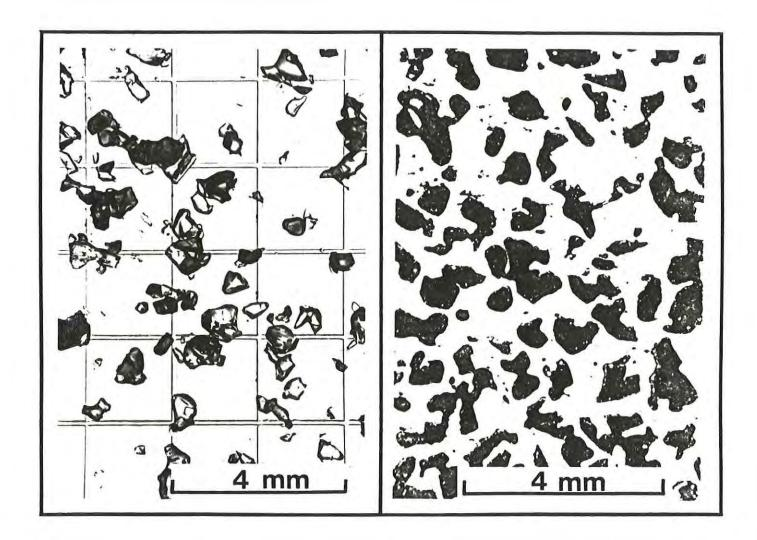
Figure 1a. Photomicrograph of disaggregated grains from a snow sample collected at middepth in a 1.5 m subalpine snowpit at Sunshine, Alberta. Sample density is 375 ± 5 kg/m³. Crystals exhibit faceted and rounded morphology.
